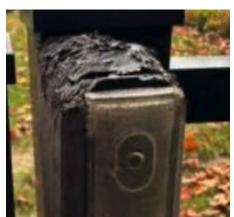
2. Get a T10 Torx Security bit and unscrew the screw on the front of the lock. Once the screw is removed, the front will come off (from the bottom area where the screw was).
